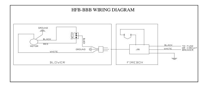
NOTE: THE JB1 JUNCTION BOX SHOULD BE INSTALLED AND THE RECEPTACLE WIRED TO THE ELECTRICAL SYSTEM OF THE STRUCTURE AT THE TIME OF INSTALLATION OF THE FIREBOX IF THE HFB-BB BLOWER IS TO BE USED.
