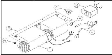
If any of the original wire must be replaced, it must be replaced with 105C rated wire gage equal to original wire's gage.
