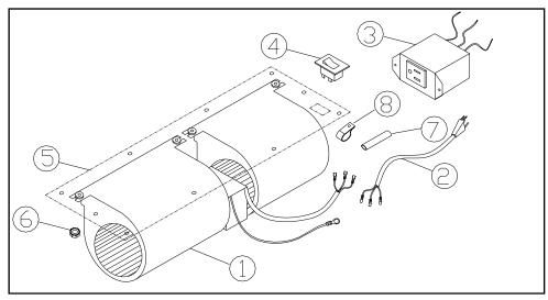
If any of the original wire must be replaced, it must be replaced with 105C rated wire gage equal to original wire's gage.
