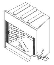
Replace with HFB-B blower assembly by first plugging power cord into receptacle located to the right under the hearth pan. Using the same ten screws, secure blower cover plate to the hearth pan.
