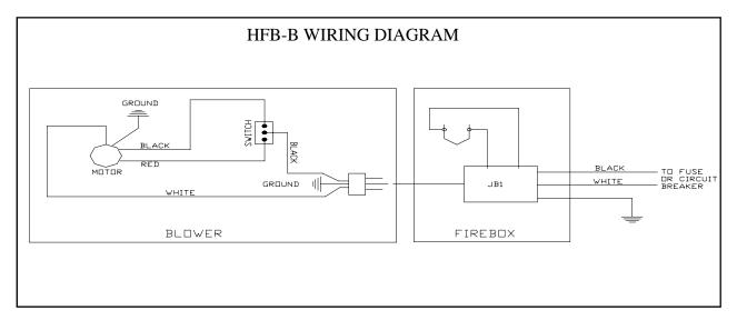
NOTE: THE JB1 JUNCTION BOX SHOULD BE INSTALLED AND THE RECEPTACLE WIRED TO THE ELECTRICAL SYSTEM OF THE STRUCTURE AT THE TIME OF INSTALLATION OF THE FIREBOX IF THE HFB-B BLOWER IS TO BE USED.
